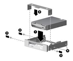
replacing the diskette drive adapter on the 8000 series
